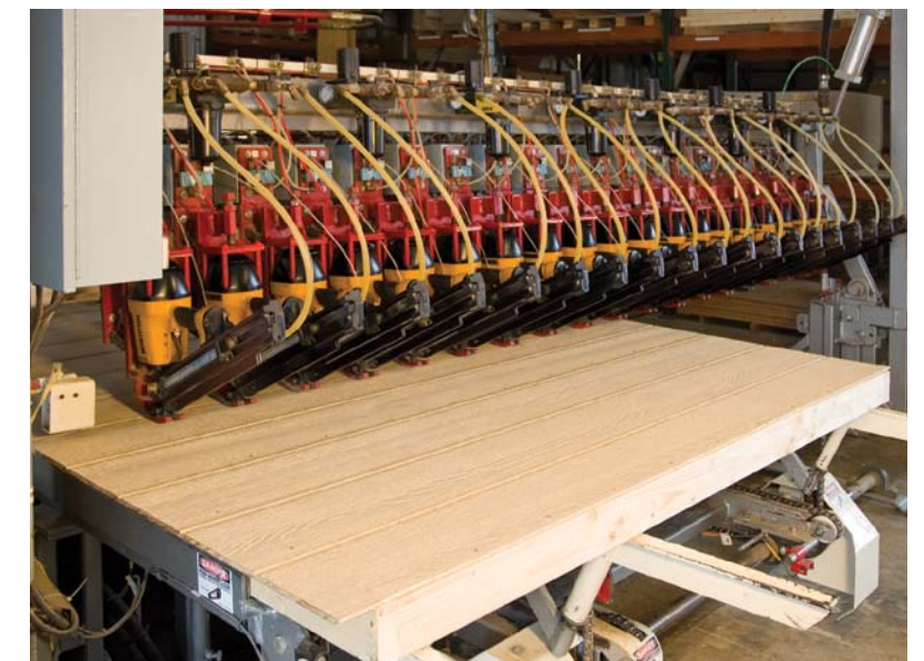
Panelization wastes less lumber; creates stronger, straighter, tighter walls; and goes together quickly with less site disturbance. Overall, it’s a better process than stick building.
