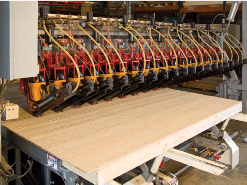
Panelization wastes less lumber; creates stronger, straighter, tighter walls; and goes together quickly with less site disturbance. Overall, it's a better process than stick building.
